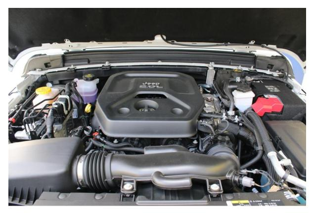
There's some new age stuff under the bonnet too, with this iteration of the Wrangler featuring a 2.0-litre turbocharged petrol engine that produces 268hp and 400Nm of torque. It does fairly well performance-wise, with enough grunt to help it move along at a decent pace despite the car's size, and the unit doesn't feel at all strained or stretch when you get going.
