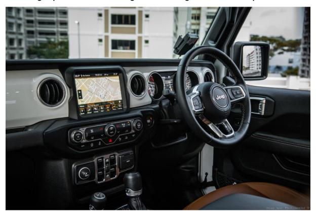
Seated close to the upright windshield, front occupants face a narrow squared-off dashboard punctuated by round air vents and chunky switches for the climate-control system, power windows, and infotainment. Every feature is a physical button, which may look outdated in today's digitalised world, but I am all for it if it benefits usability.
