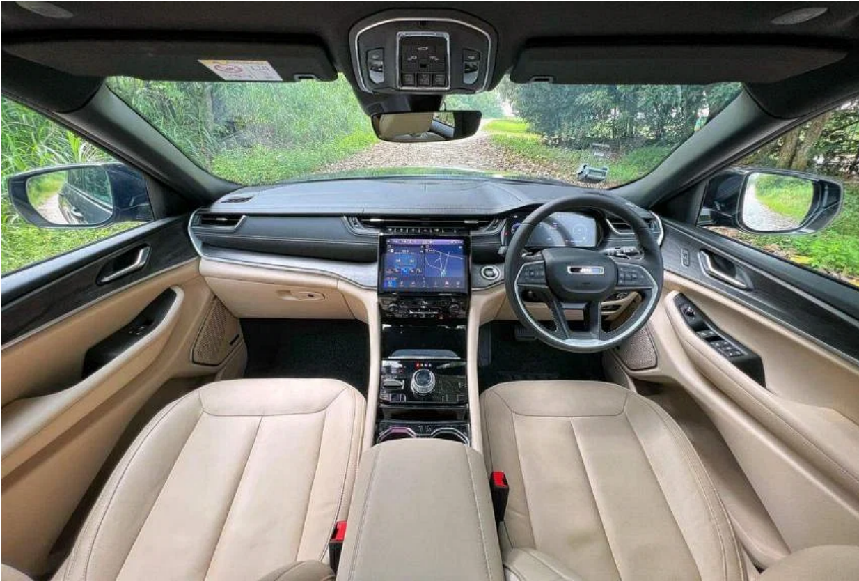
Posh and polished: A rotary gear selector, a 10.1-inch infotainment touchscreen, and digital instrumentation with head-up display. ST PHOTO: KEVIN LIM
