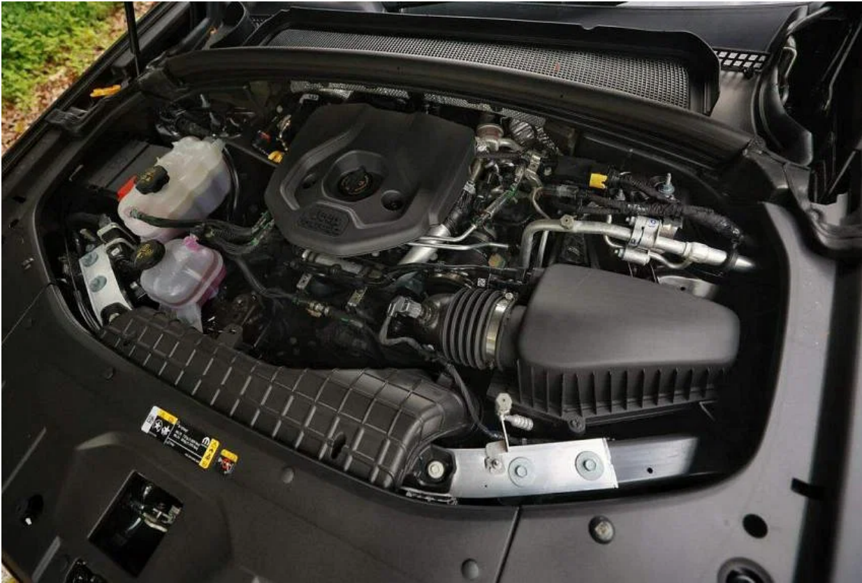
Beneath the bonnet: A 2-litre turbo engine which outguns Jeep's previous normally aspirated 3.6-litre V6. ST PHOTO: KEVIN LIM
